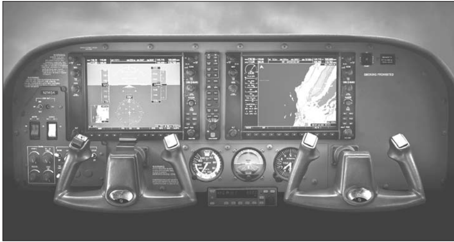
The full G1000 in a Cessna 172 showing relative positions of PFD, MFD and standby instruments.
