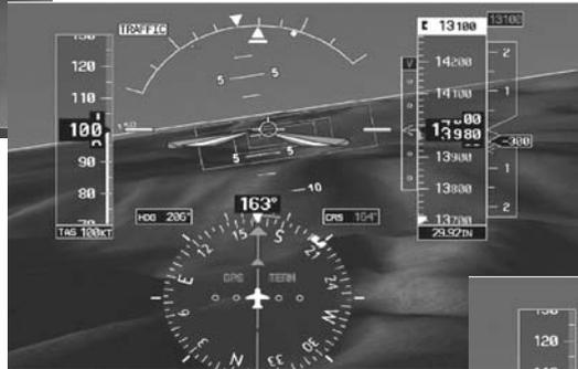
*Some of the abilities of synthetic vision: joining Highway In The Sky (upper left - the goal is to fly through the rectangles); top of descent for the GPS-C into Aspen, Co. (above), at the MAP for runway 15, Aspen (right).*
