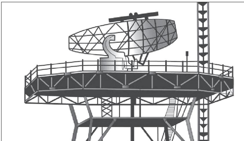
An ASR-9 radar. The top, horizontal bar is the Secondary Surveillance Radar. The lower “hog trough” antenna is the Primary Surveillance Radar.
