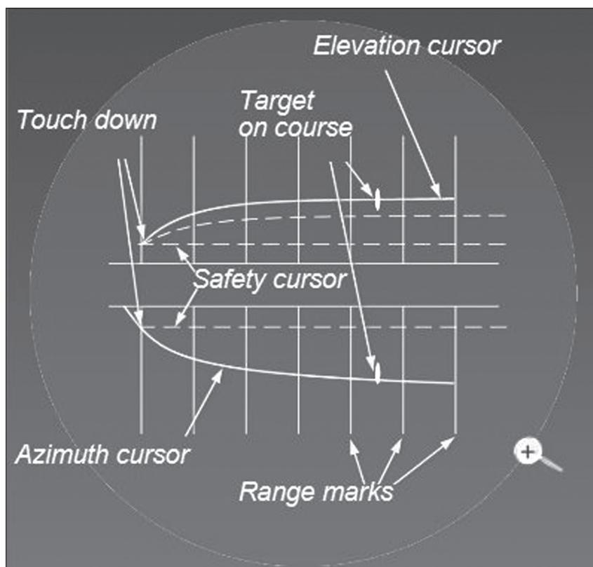
*Precision Approach Radar screen presentation. The upper (Elevation Picture) portion of the display gives a side view of the landing approach down to the runway touchdown point with an imaginary line for reference. It shows altitude determined by the height-finding radar. The lower (Azimuth Picture) portion of the display shows azimuth determined by the PAR's horizontal sector scanning. Both pictures show distance.*
