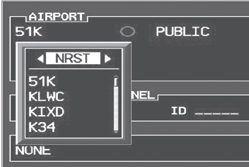
Figure 1. Hitting PROC brings up the nearest airports regardless of whether they have an Instrument Approach PROCEDURE.
