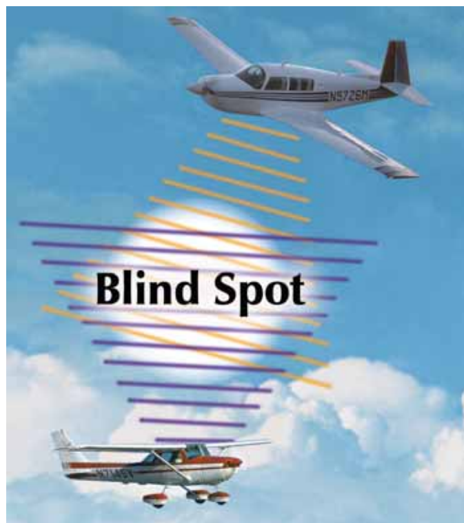
When scanning for traffic, the pilot must be aware of the blind spots that can be created by aircraft design.
